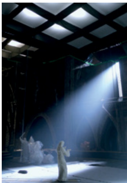
SkyPanels in light boxes, providing a clean, soft, controllable top light on the great hall set.
